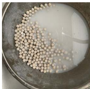
Figure 6: Neutralization media that has been rinsed with clean water
