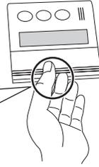
If it does not come off, insert a flat head driver into the notch at the bottom of the cover and slightly twist it to remove.
